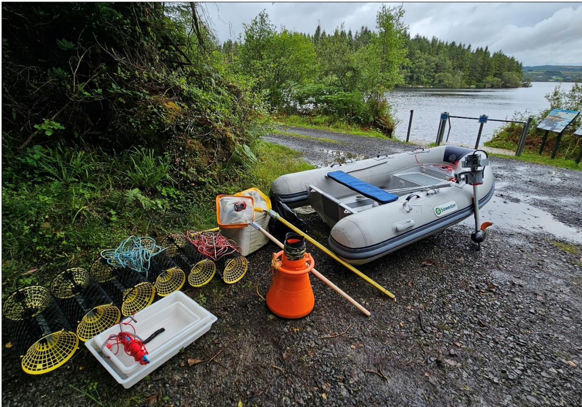
Plate 2.1 Crayfish traps prior to deployment, with sweep net and bathyscope to aid with physical and visual searches
