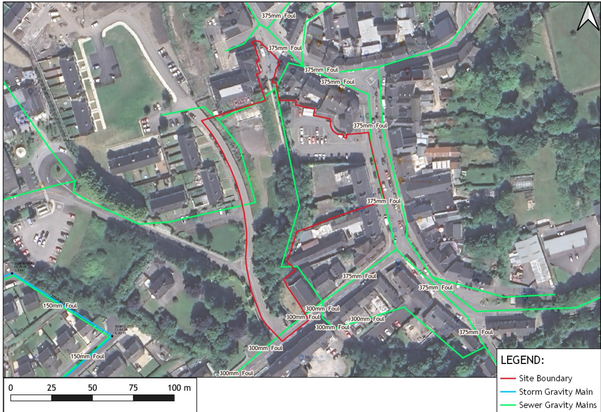
Figure 3-4: Existing Public Drainage in the vicinity of the site (source: Irish Water)
