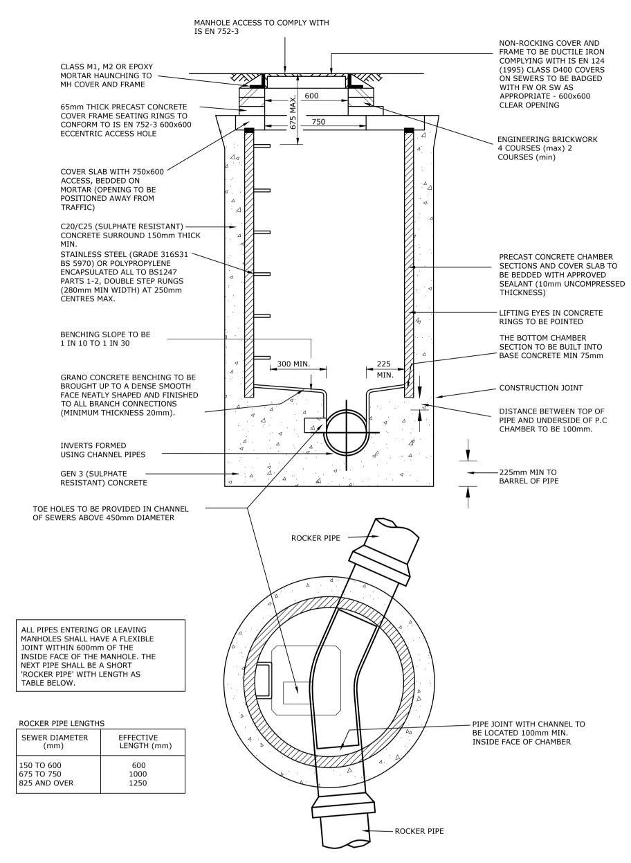
TYPICAL MANHOLE DETAIL FOR SEWER DEPTH TO SOFFIT UP TO 3.0m
