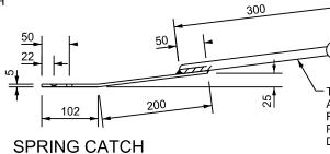
THIS LEVER MAY BE FORGED AS AN ALTERNATIVE TO THE FABRICATED ONE SHOWN, PROVIDED IT MAINTAINS THE **DIMENSIONS GIVEN**
