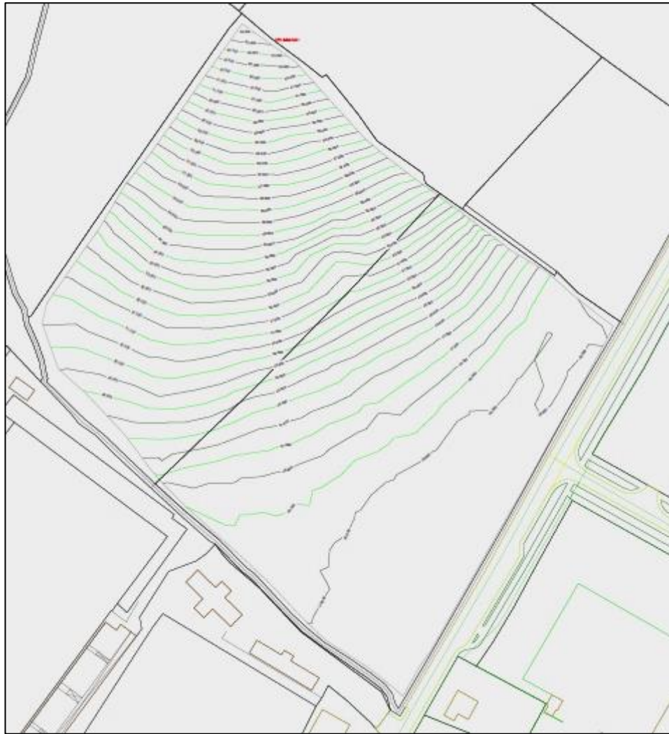
Figure 3 Contour Survey of Site
