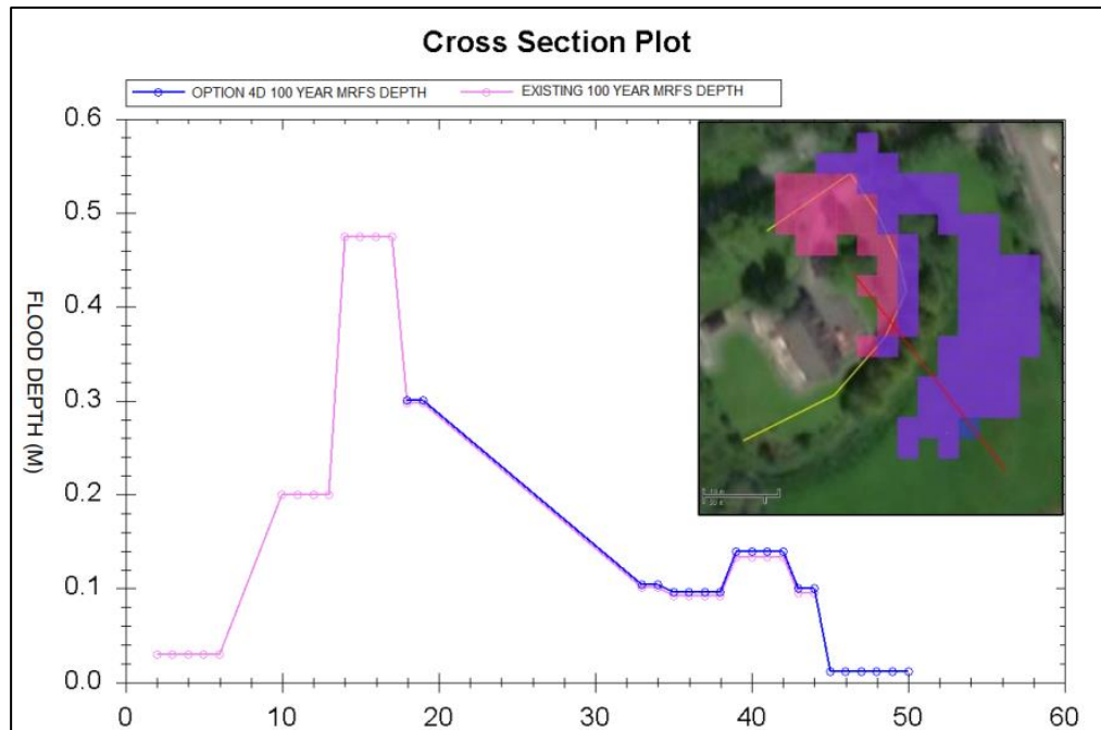
Figure 2-7: Residential Property No.2 Predicted water levels of the Ardakup More floodplain at the highlighted cross section (1 in 100-year MRFS)
