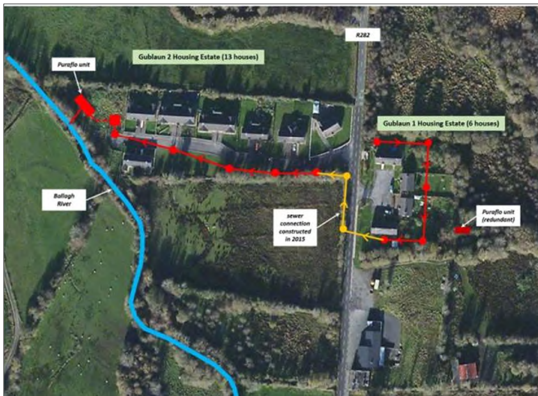
Figure 4.1 Existing Sewage System Site (Gublaun 1 on the east and Gublaun 2 on the west)
