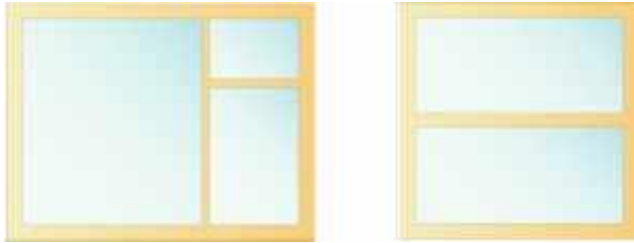
Fig. 3.5: Inappropriate Window Subdivisions
